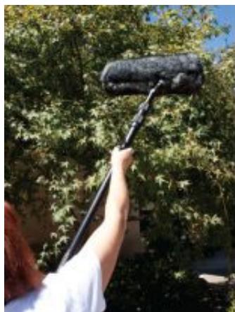
A boom pole and shotgun mic will require a person to operate, but can get quality sound from many different sources. Blimps are cages covered in fur-like material that encase the mic and should be used to mask heavy wind noise.
