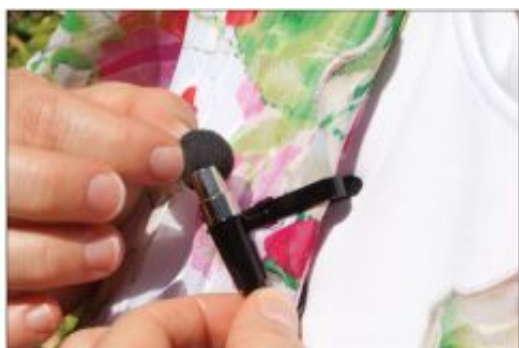
Attaching a lavalier to clothing can be a great option for getting a mic close to your talent. When outdoors, add a small windscreen to block wind noise.
