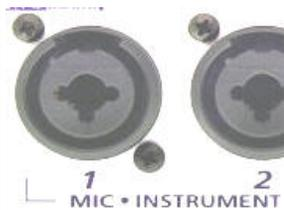
Note that the combo jack allows you to connect either XLR -or- 1/4" cables. (The 1/4" connection might either be HiZ (high impedance, i.e., "instrument level" like guitar or "line level" like keyboards, tape decks, external processors, etc.)
